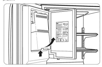
3. To reinstall the in-door ice bank, slightly slant the bin during replacement to avoid contact with the icemaker.
